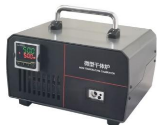
ETC-150 Miniature dry well furnace
